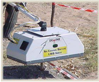
Radar head including the RF-electronics, the fast digital pre-processing and the antenna array.
