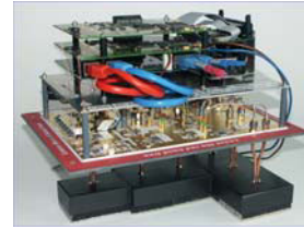
One complete module Radar module: below – the antenna array (courtesy I.D.S. Ingegneria dei Sistemi S.p.A, Pisa, Italy); middle – RF-electronics (3 transmitters and 4 receivers); top – digital pre-processing, power supply, data interface, operational control
