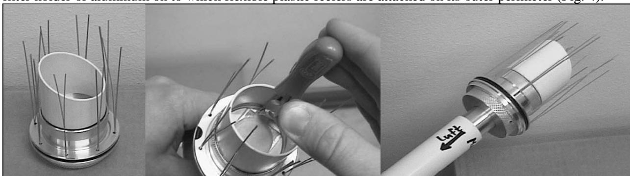
**Fig. 4 End piece of the sweeping collector**
