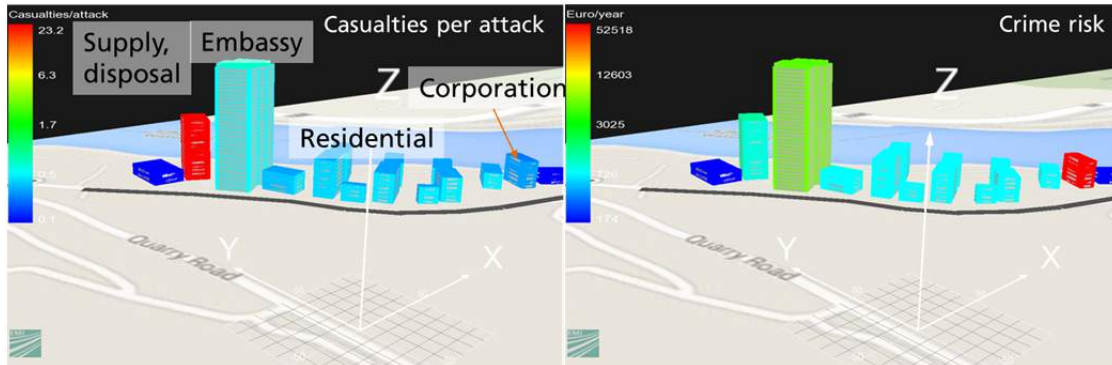
Fig. 4, Left: 3D Model of Water Haven with types of buildings and empirical consequences in terms of injuries + fatalities per attack; Right: Empirical monetary risk analyses for crime.
