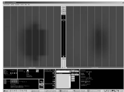
Fig. 4 Signals for stacked coils providing the basis for depth estimation
