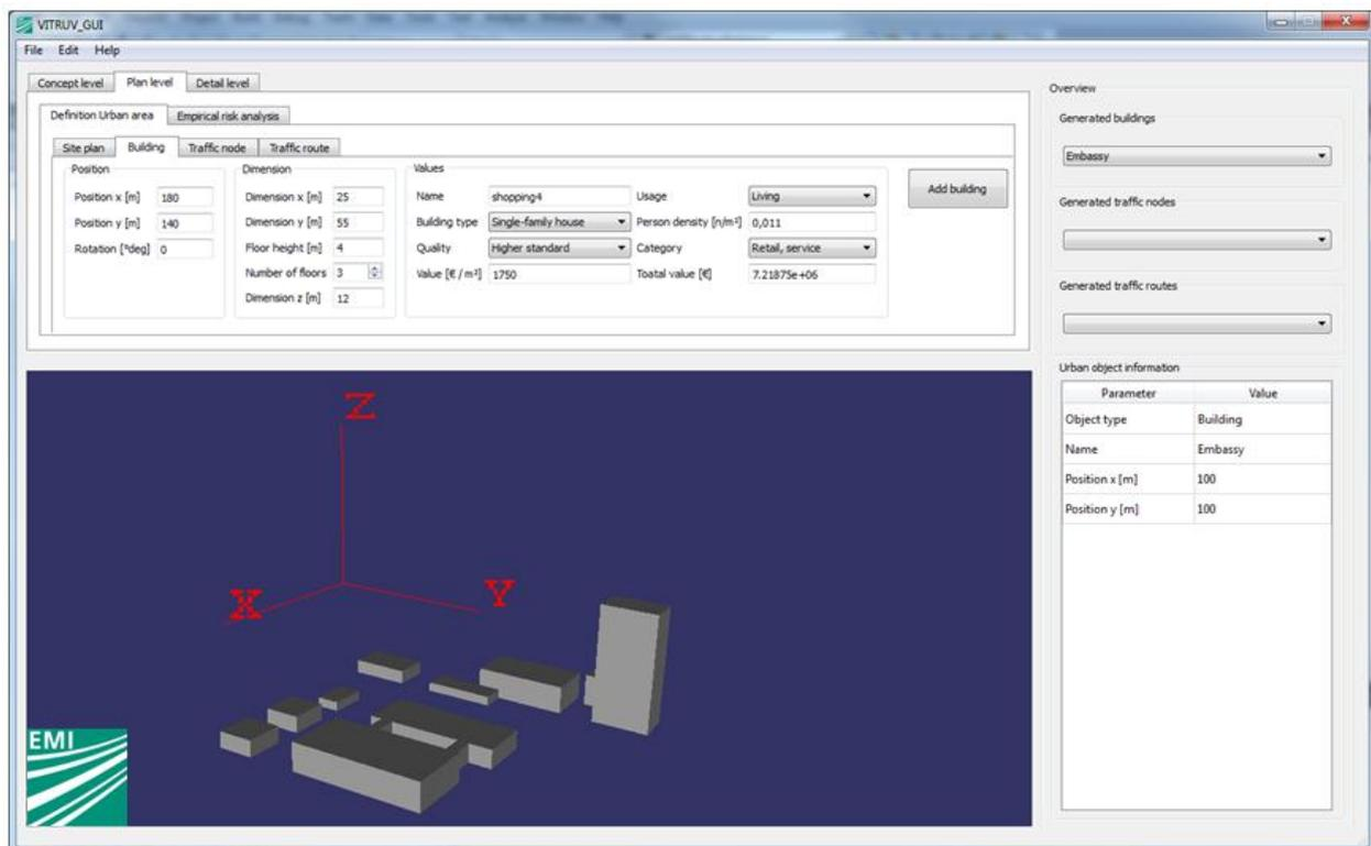
Figure 6: Window application of the VITRUV tool for plan and detail level.
