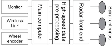
Fig. 4. Schematics of the trough wall imaging radar
